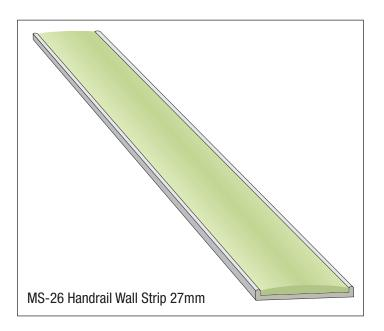
The MS-26 Handrail Wall Strip is designed to ensure visibility of handrails in escape routes to meet NZBC Clause F6 "Visibility in Escape Routes". The guidance strip is fitted to the wall above the handrail and will be effective in all light conditions including during failure of the main lighting.
